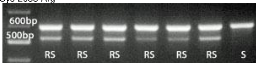
Figure 1. Genomic PCR based marker analysis of the ACCase mutations shows only homozygous susceptible (S) and heterozygous resistant (RS) genotypes for the: (a) 1781, (b) 2078 and (c) 2088 mutations detected in the ACCase-inhibiting herbicides surviving plants.
